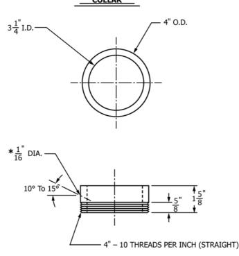
Note 1—The  $\frac{1}{16}$ -in. (1.6-mm) diameter hole is for a Luxtron MIW temperature sensing probe. Number of holes and location may vary by application.
